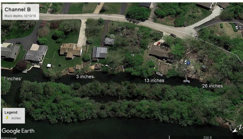
Figure 2 Post-Treatment of Muck depths Fall 2019 in Channel B.
